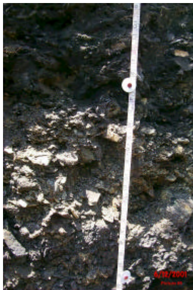
Picture #5, Pit #1 west side Iron and Sulfur precipitation.
